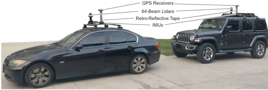
Fig. A5. Vehicles used to collect experimental data. Each vehicle is equipped with NOVATEL GNSS receiver, OS1-64 LiDAR, and STIM 300 tactical grade IMU. Relative pose measurements are obtained by detecting retroreflective tape attached on each sensor suit mounted on each vehicle.
